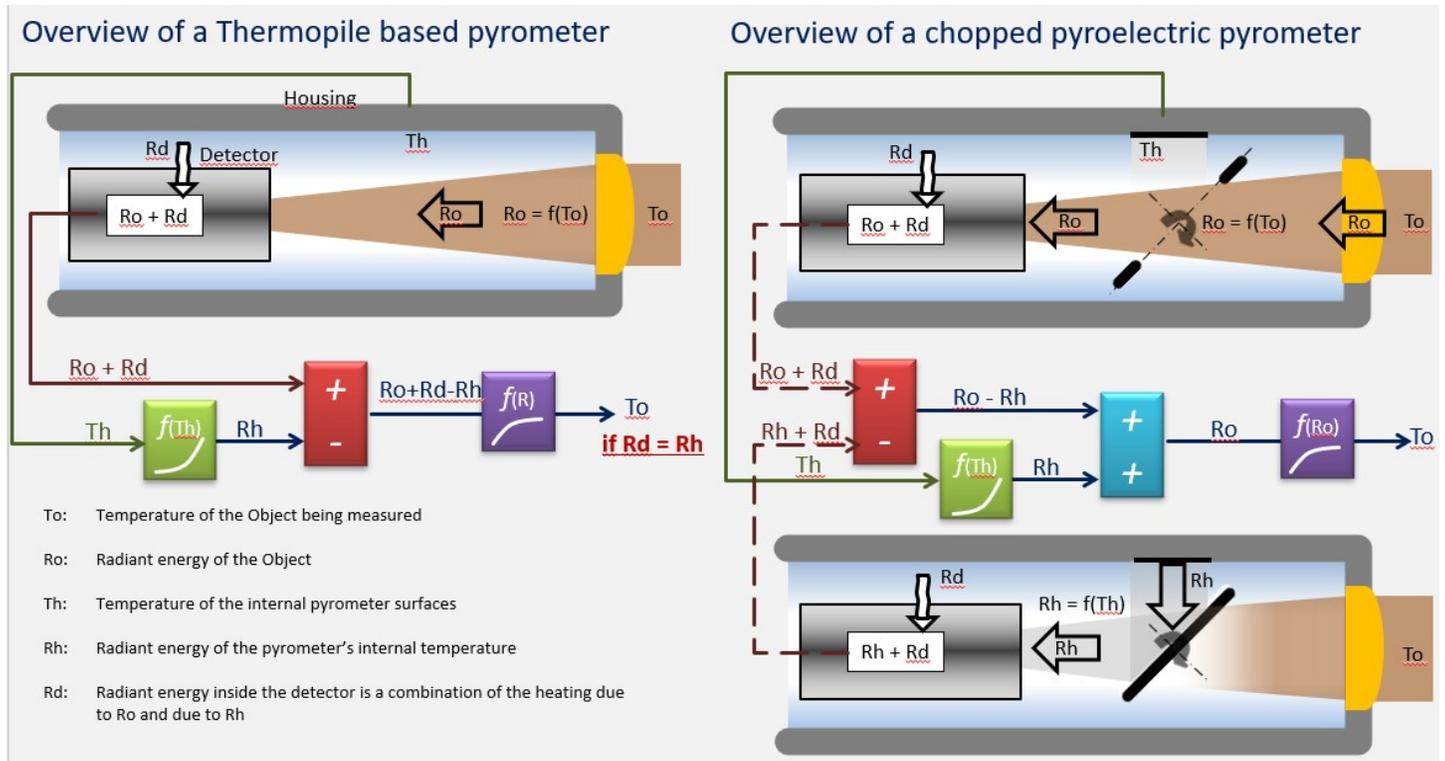
During the short chopping cycles, which are normally in the millisecond range,  $T_h$  and  $R_d$  do not change. The bias is thus eliminated completely and substituted using  $R_h$ , which is measured well within a specified reference accuracy of  $<0.5\text{ }^\circ\text{C}$  ( $0.9\text{ }^\circ\text{F}$ ) over the permissible ambient temperature range.
